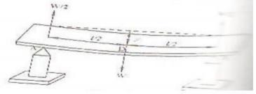
The beam may be considered as two cantilevers, whose free end carries a load of W/2 and fixed at the point 'D'.
