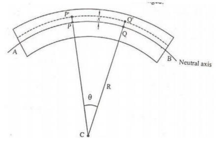
Let PQ be the chosen from the neutral axis. If R is the radius of curvature of the neutral axis and  $^{\theta}$  is the angle subtended by it at its center of curvature'C' Then we can write original length
